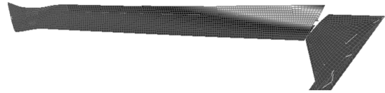
Fig. 7 Aftwing twist-down configuration with spanwise slit.
